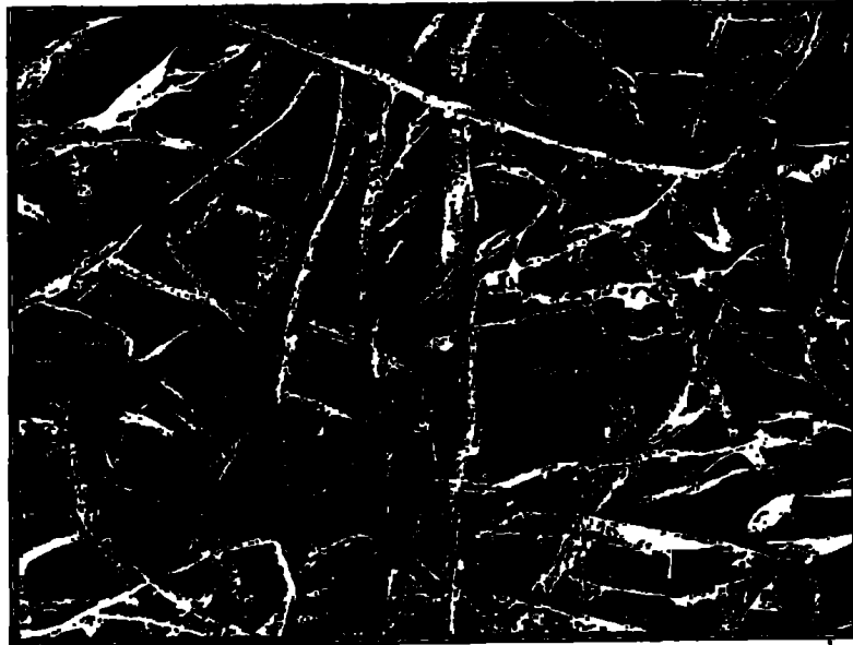
FIGURE 5 EXPERIMENTAL AIRLAD STRUCTURE - TREATED SURFACE Hitachi Scanning Electron Microscope (BSE image) Mag. 80X
