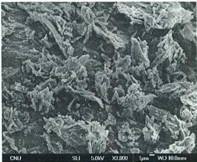
Fig. 4. SEM micrograph of unprocessed atorvastatin particles, crystalline (×3000).
