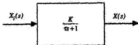
FIG. 8-4 First-order transfer function.
