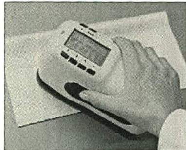
A portable sphere spectrophotometer measures the color of textile samples and other materials where the product's appearance is critical for buyer acceptability.
