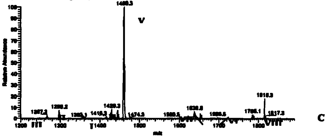
Fig. 40. Mass spectra of impurity Iso B0: A) full scan 1000-2000 amu (monocharged ions), B) full scan 600-1000 amu (doublecharged ions), C) fragmentation of [M+H]^+ ion.
