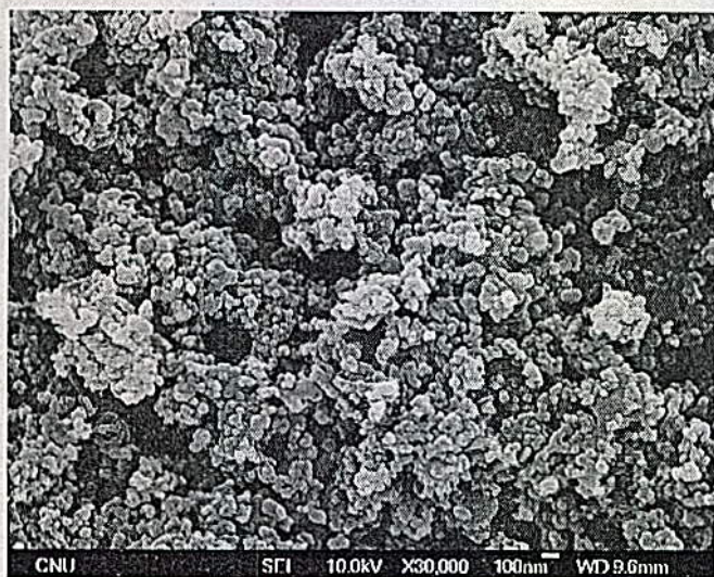
Fig. 6. SEM micrograph of SAS processed amorphous atorvastatin calcium precipitated from a tetrahydrofuran solution ( \times 30,000 ).
