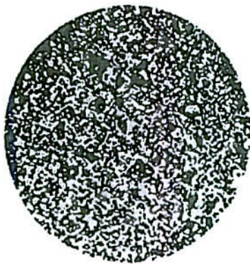
Figure 3-4B. Cement + water + dispersant.
