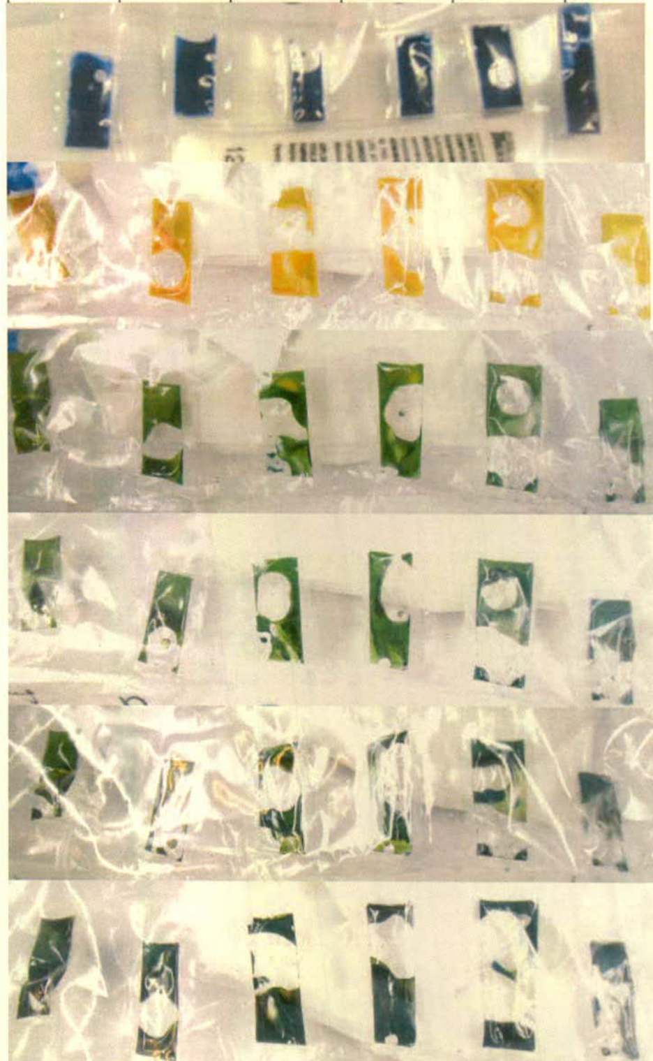
Figure 6. Colour changes of indicator with 2.0 g/10 ml microcrystalline cellulose added (pH adjusted).
