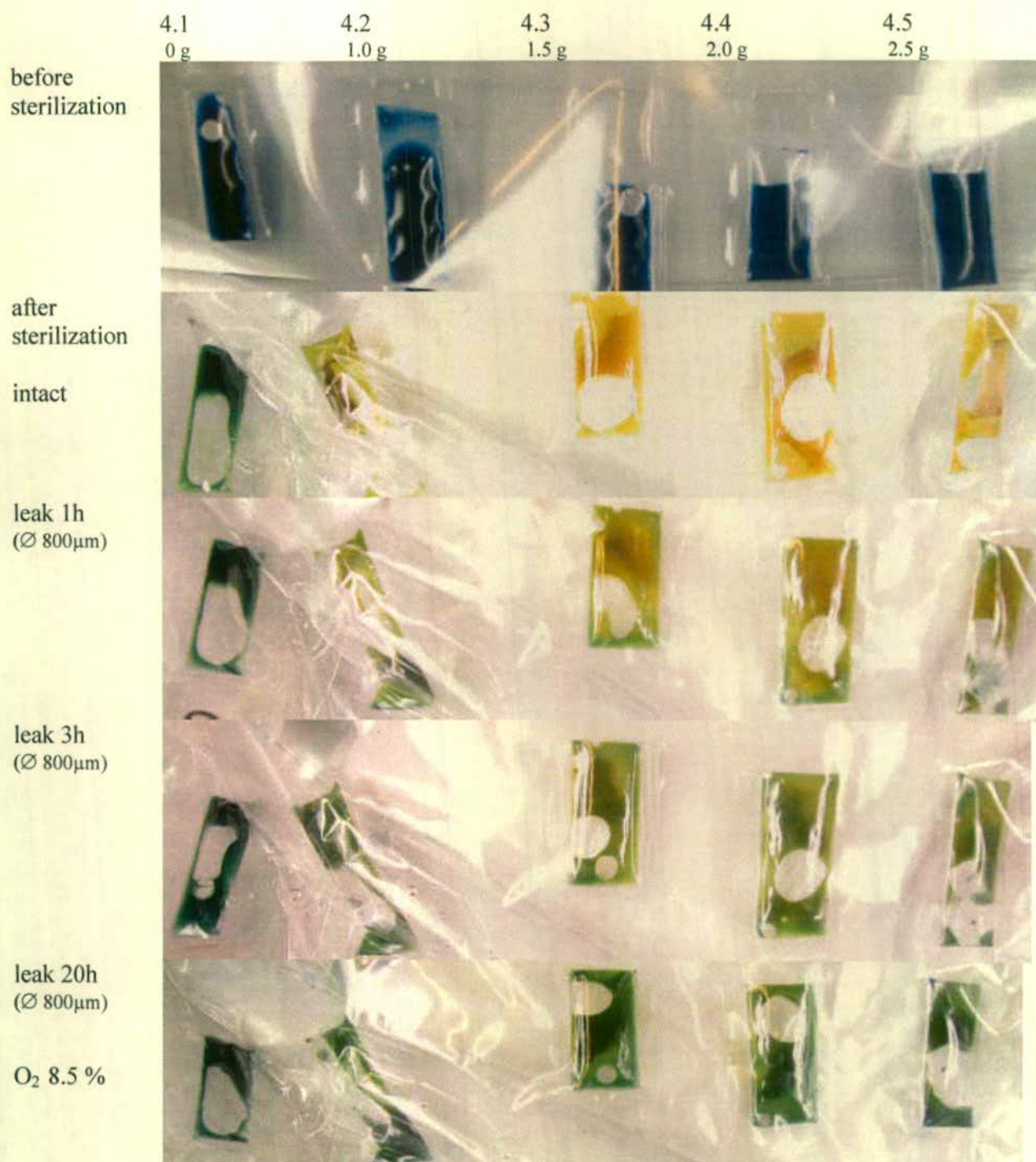
Figure 7. Colour changes of indicators with different amounts of microcrystalline cellulose added. 0.13 M sodium pyrophosphate solution was used. pH not adjusted.
