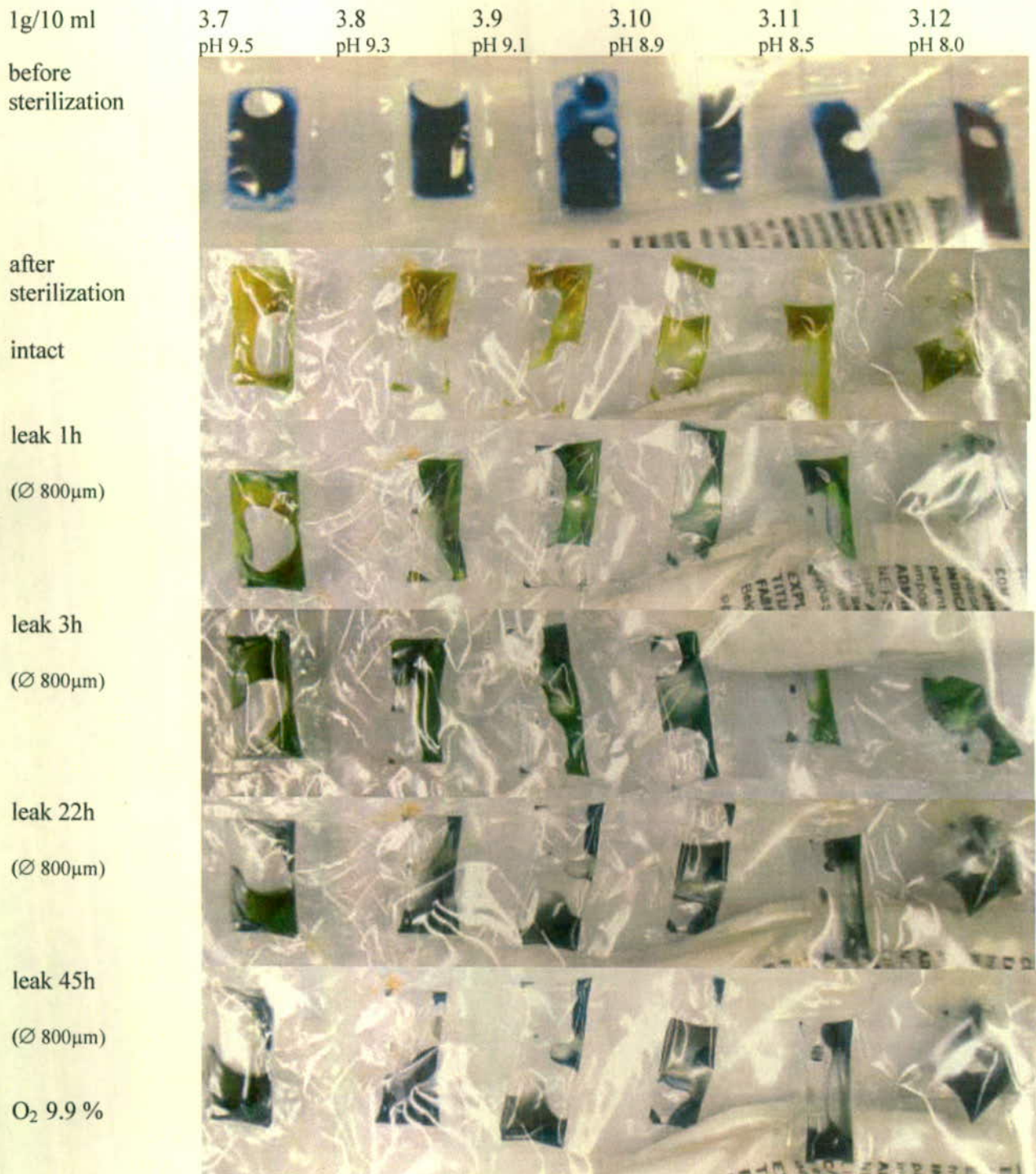
Figure 4. Colour changes of indicator with 1 g/10 ml microcrystalline cellulose added (pH adjusted).
