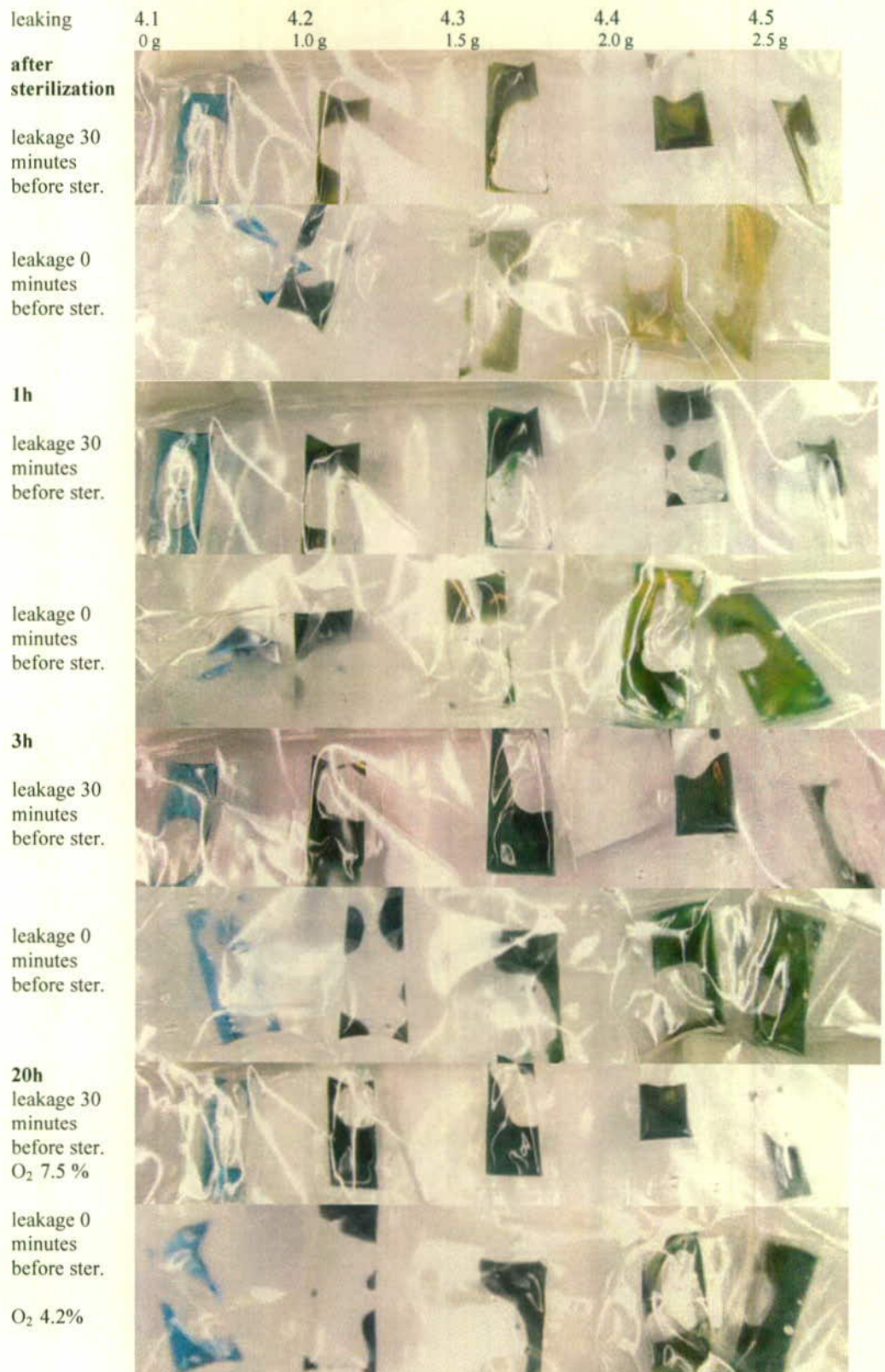
Figure 8. Colour changes of indicators in leaking packages. Leakage was made to the packages either 30 minutes or 0 minutes before sterilization.
