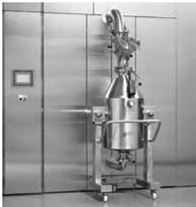
Figure 26-17. Examples of Rubber Stopper Preparation Systems that clean, siliconize, and depyrogenate stoppers. (Courtesy of Getinge.)
