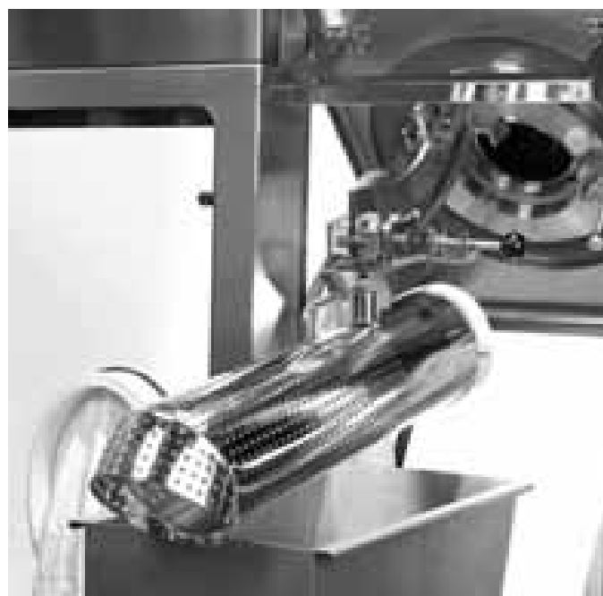
Figure 26-17. Examples of Rubber Stopper Preparation Systems that clean, siliconize, and depyrogenate stoppers. (Courtesy of Getinge.)
