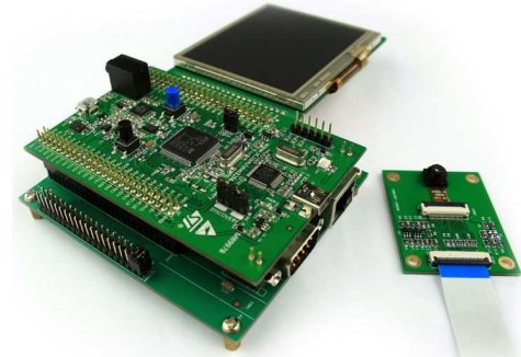
Fig. 1: Discovery Kit: main board, base board, camera and display
