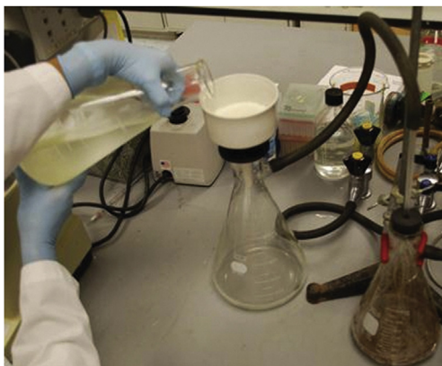
FIGURE 3.1 After centrifugation of the culture to remove the majority of the bacteria, filtration is used to remove residual bacteria from the supernate. Reprinted with permission from Crowley, T. E., & Kyte, J. (2014). Experiments in the purification and characterization of enzymes: A laboratory manual. Amsterdam; Boston, MA: Elsevier/AP, Academic Press is an imprint of Elsevier. Retrieved from < https://lccn.loc.gov/2014395777 > .
