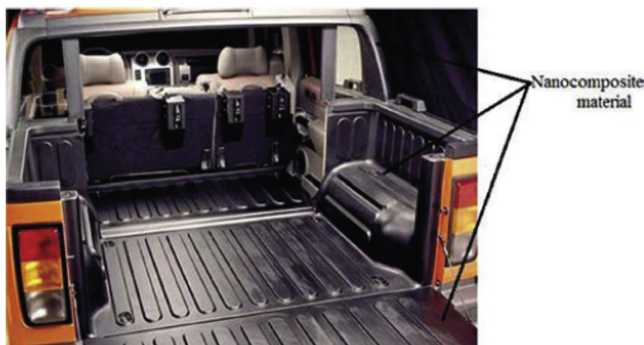
Fig. 11. Use of nanoclay-polymer composite materials on a truck bed. (taken from Reference [156].)
