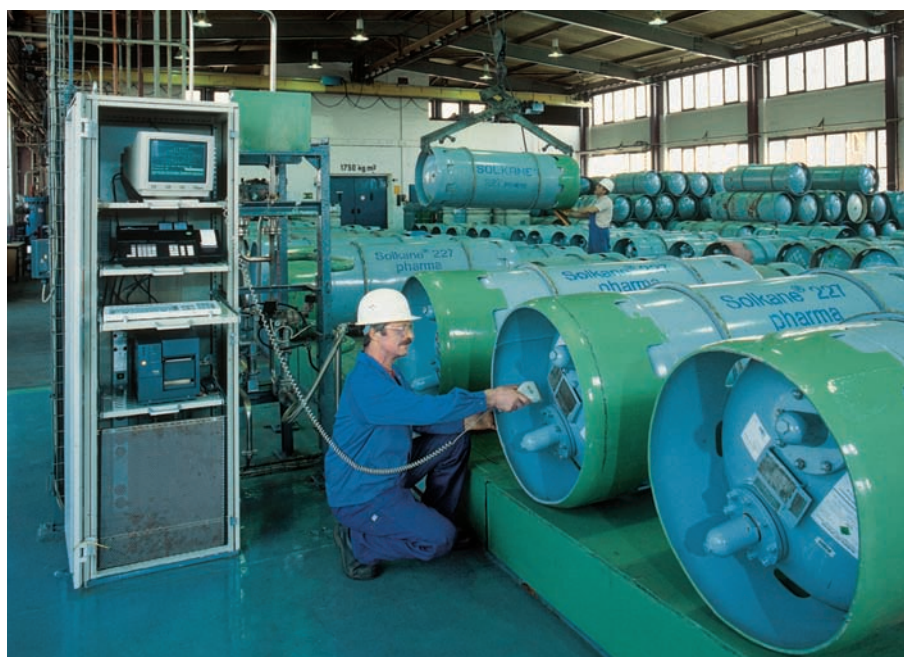
Fig. 9: Electronic bar code scanning of SOLKANE™ 227 pharma one tonne cylinders for identification and traceability
