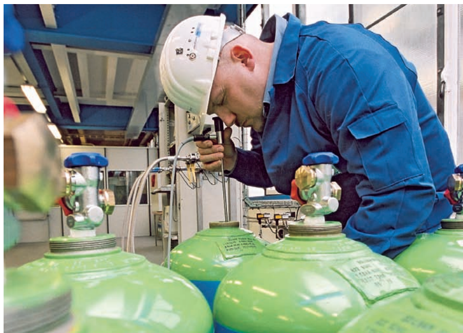
Fig. 7: Visual inspection of dedicated SOLKANE™ 134a pharma cylinders as part of Daikin's quality control
