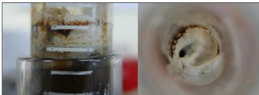
Fig. 3. Precipitate formed after gravity drainage flooding test (GDFT) at room temperature conditions.
