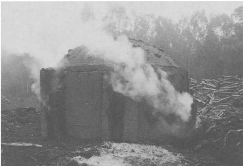
Photo 6 A Brazilian beehive brick kiln in full operation. (Photo W. Emrich)
