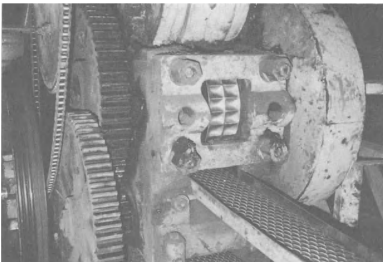
PHOTO 14 A charcoal briquetting press. Two rows of moulds can be seen and the wire belt. (Photo W. Emrich)
