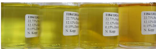
Figure 6: Solutions with 0.15 % citric acid at 5, 25, 40, 60 °C after 1 month storage.
