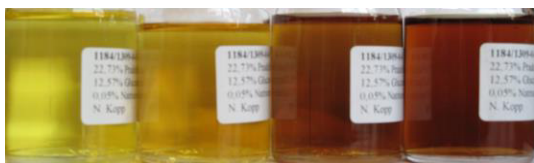
Figure 2: Solutions with 0.15 % sodium ascorbate at 5, 25, 40, 60 °C after 1 month storage.
