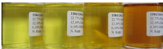
Figure 3: Solutions with 0.15 % glutathione at 5, 25, 40, 60 °C after 1 month storage.
