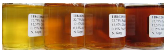
Figure 1: Solutions with 0.15 % ascorbic acid at 5, 25, 40, 60 °C after 1 month storage.
