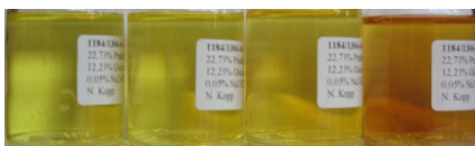
Figure 4: Solutions with 0.05 % sodium EDTA at 5, 25, 40, 60 °C after 1 month storage.
