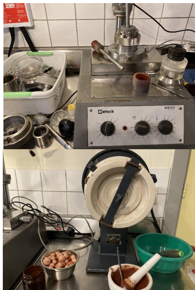
Fig.10: Up-scaling in lili's lab: mortar and pestle; high speed micro mills: sample preparation for analysis without contamination, fineness, homogeneity, short time, versatility, speed selection, different grinding media; ceramic jar ball mills.
